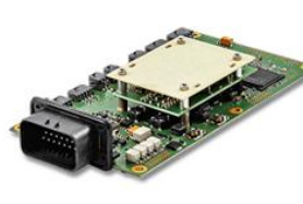
Battery Management System
