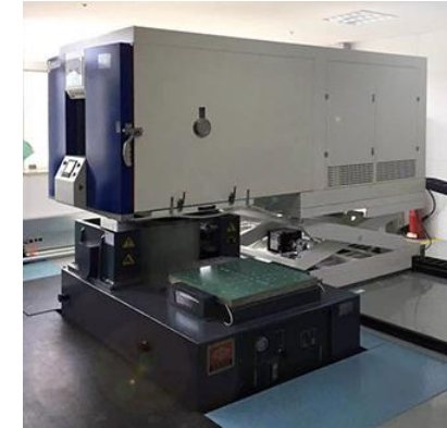
AGREE Test Chamber (Temperature Humidity and Vibration Test)
